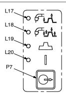
Always check and set a trigger mode. If trigger mode is undefined for a welding process, select the desired mode.
